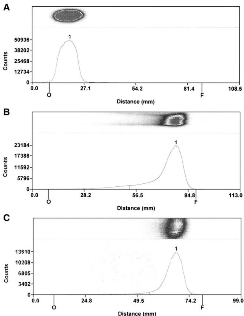
Fig. 1. Illustrative example of the quality control of  $[^{68}\text{Ga}]$ -EDTMP. (A) Free  $[^{68}\text{Ga}]$ -gallium. (B)  $[^{68}\text{Ga}]$ -EDTMP after 5 min. (C)  $[^{68}\text{Ga}]$ -EDTMP after 300 min (O=start, F=solvent front).
